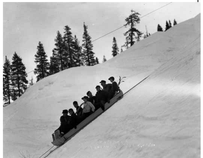
Top and bottom: the UpSki at Auburn Ski Club - one of the earliest ski lifts. Center: an example of an UpSki or Boat Sled.
